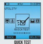
Start a test on a single cell or monoblock without setting up a site.
