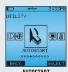
**AUTOSTART** Set the tester to activate a test process on contact.
